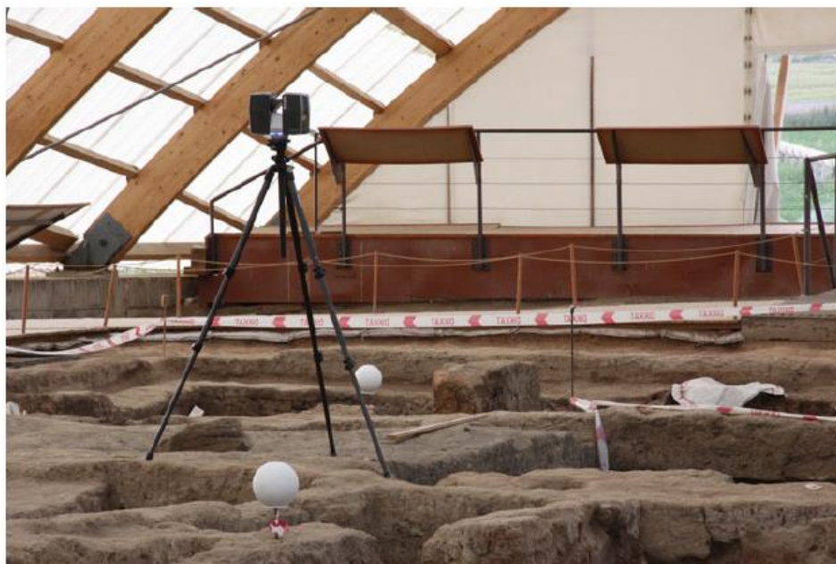
Figure 2. Example of cyberarchaeological application for field data collection: FARO Focus 3D S120 scanning Neolithic buildings in the North Area of Çatalhöyük's East Mound. Source: Lercari (2016, p. 18, fig. 8).
